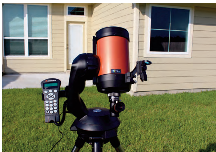
Image 6 - A close up view of the NexStar 5se telescope and mount. The author acquired a removable 3D-printed bracket to hold the hand controller at a better viewing angle while using the telescope.
