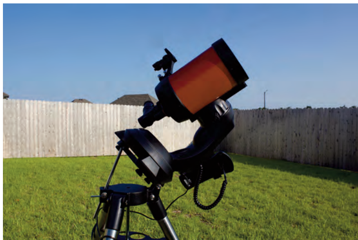
Image 15 - The NexStar 5se in equatorial mode is polar aligned by pointing the hinged side of the wedge due north and adjusting the latitude scale to the correct latitude.
