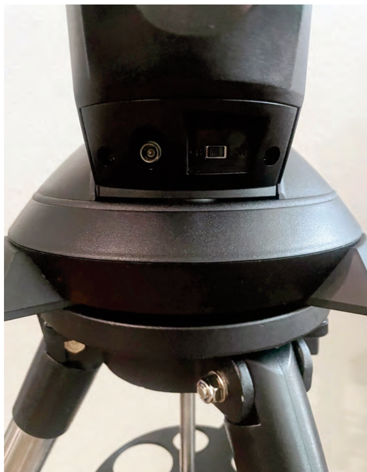
Image 10 - The on/off switch is at the very bottom on the mount's arm next to a jack to attach an external 12-volt power supply to use in lieu of AA batteries.
