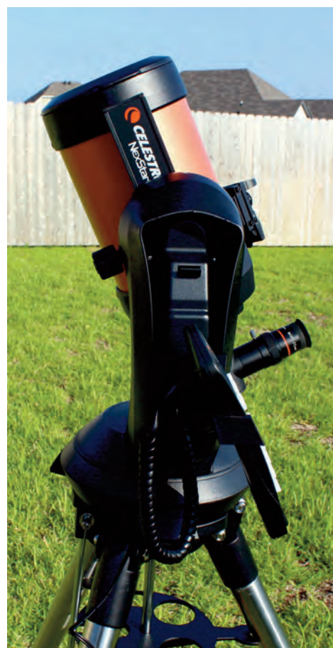
Image 8 - The hand controller can be stored in the outside portion of the mount's arm when not using the add-on 3D-printed bracket.
