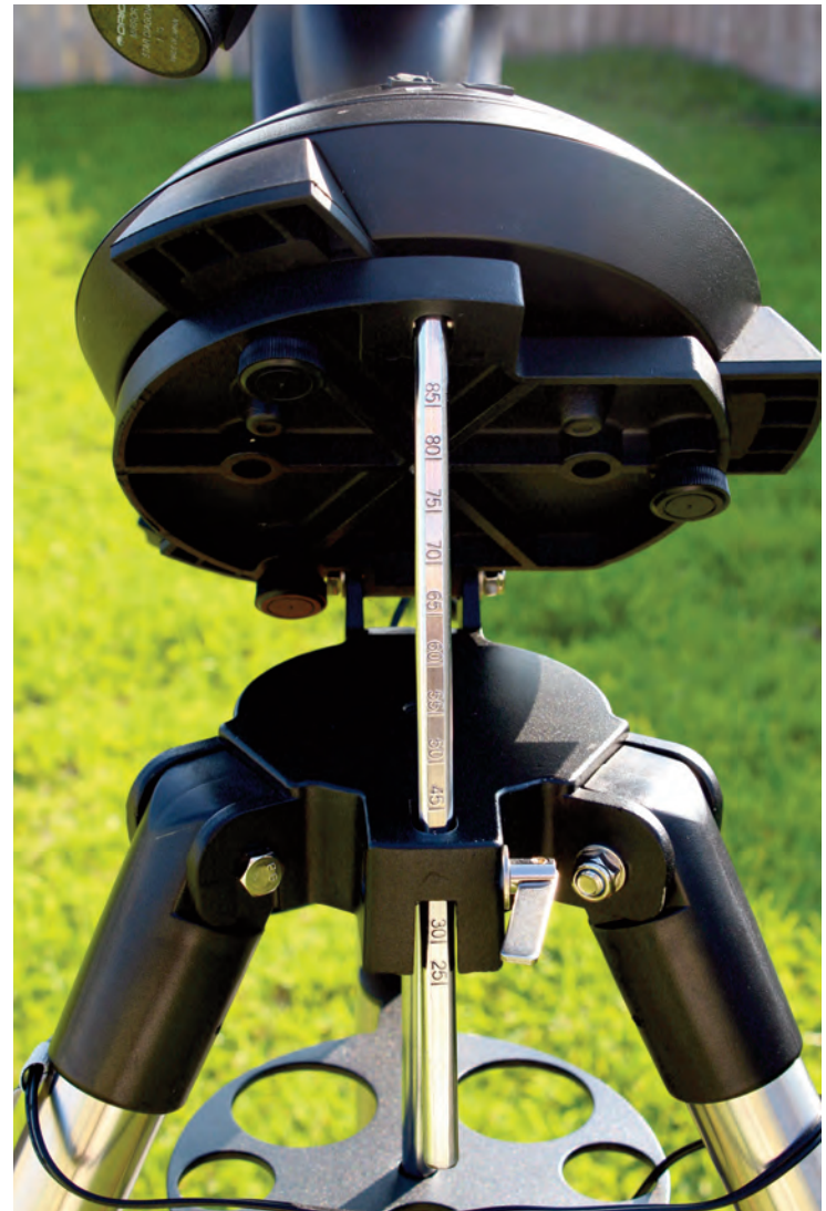
Image 14 - The mount has a built-in equatorial wedge with a latitude scale. This allows the telescope to operate in equatorial mode.
