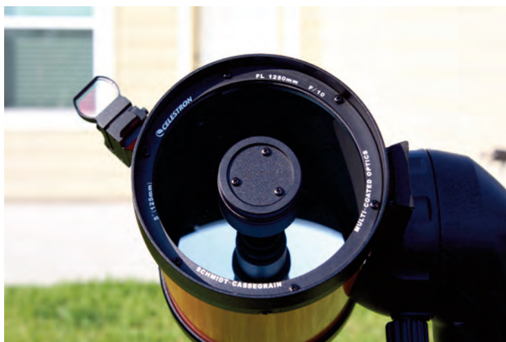
Image 11 - Inside view of the optical tube assembly. The corrector lens assembly holds the secondary mirror in place. The three Phillips screws on the secondary assembly are for collimating the optics.
