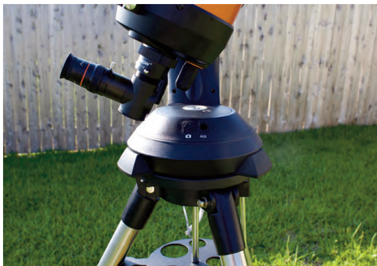
Image 9 - There are two ports on the mount base. One is for attaching Celestron auxiliary devices to the mount. The other port is to connect a firing cable from the mount to a DSLR camera to control the camera with the mount's hand controller.
