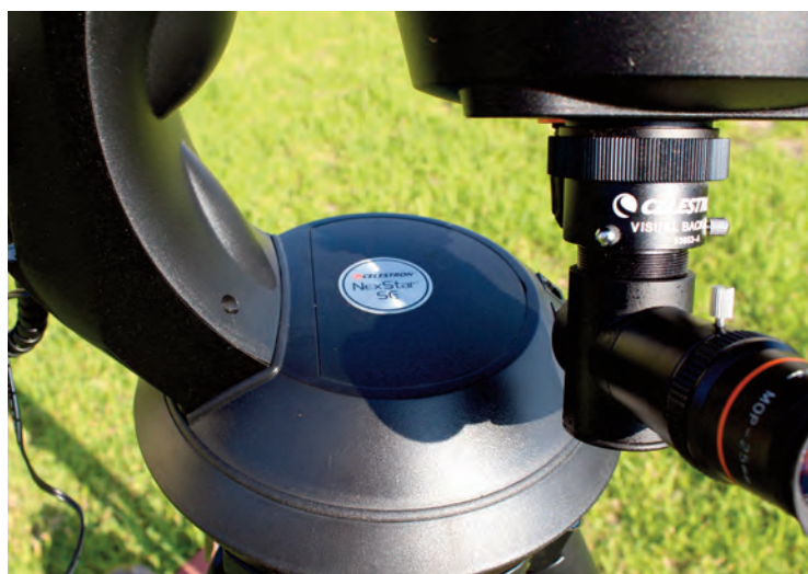
Image 7 - A removable cover on the top of the mount base has a compartment for 8 AA batteries to power the mount.
